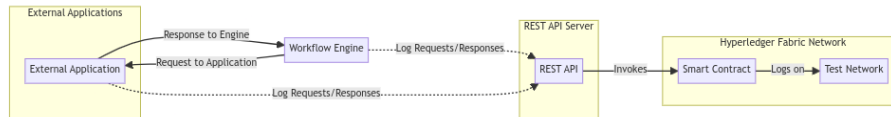
Fig. 2: Architecture of the REST API-based approach. The workflow engine initiates a process that interacts with external applications and logs these interactions through the REST API to a smart contract deployed on the Hyperledger Fabric network.
